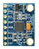
MPU-6050 Six-Axis (Gyro + Accelerometer) MEMS Motion Tracking
