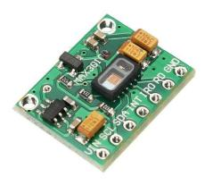
The MAX30105 Particle Sensor is a flexible, powerful sensor enabling sensing of distance, heart rate, particle detection and even the blinking of an eye. The MAX30105 has been equipped with three LEDs as well as a very sensitive photon detector. The idea is to pulse the different LEDs, then detect what shines back. Based on the reflected signature it's possible to detect different types of particles or materials (such as oxygenated blood or smoke from a fire).
